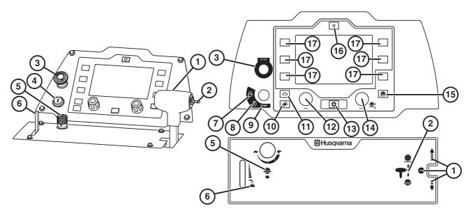
The control panel is the operator's link to the machine. From here the operator can control anything from engine rpm, cutting depth of the blade and read the current status of the engine and the machine.
