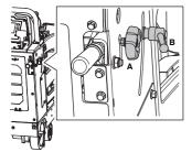
Lower the front guide and align the front guide, rear guide and the diamond blade with the line on the surface. The front guide is telescopic, adjust the length with the screws on the inside of the front guide.
