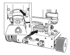
Refill the system by removing the left screw and pour oil into the tube. Look in the window and fill until the correct level is reached.
