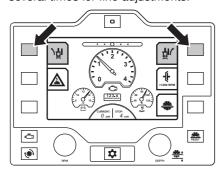
By pressing the E-track zero button on the control panel the rear axle will return to predefined center angle.
