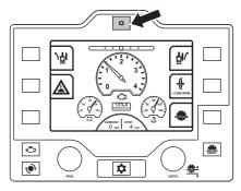
Return to previous setting by once again pressing the Etrack zero button on the control panel.  The E-track gauge on the display will indicate the present angle of the rear axle. The change is saved both if the ignition is switched off or if the machine is without power.
