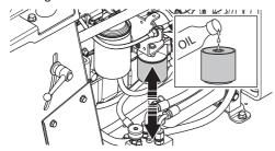
Refill the reservoir with new oil. Ensure that machine is level prior refilling.
