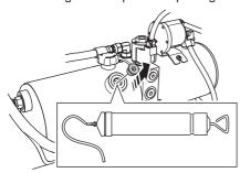
Replace the hydraulic system filter. Fill the new filter with oil and lubricate the seal with a few drops of oil prior to refitting it.
