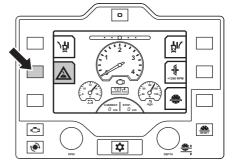
Engage the Blade clutch (if equipped) to engage the blade drive. Only at 1200rpm or less.
