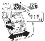
Hand tight knob. Tighten jam nut (40 Nm/30 ft-lb).
