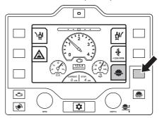
Lower the saw by pushing the Raise/lower switch on the speed control lever downwards until the blade touches the surface to be cut. This will be the reference point.
